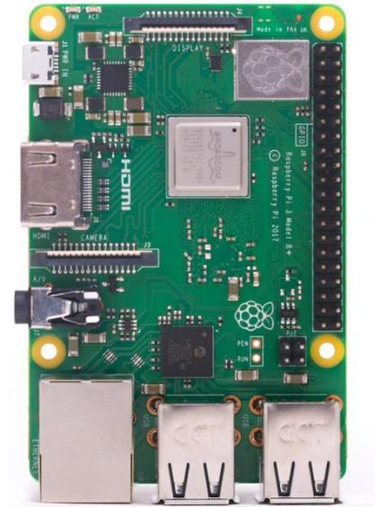
Figura 3 - Raspberry Pi 3 Model B+ Front
