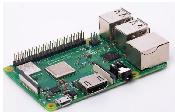
Figura 2 - Raspberry Pi 3 Model B+
