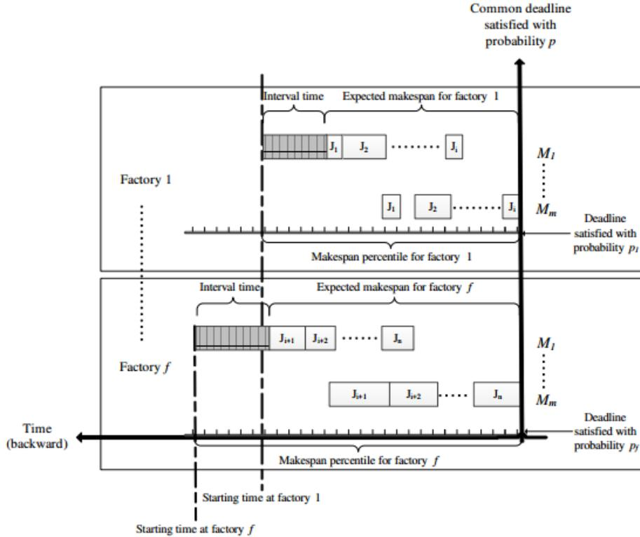
FIGURE 7.1: Starting time, expected makespan and makespan percentile in the DPFSP-ST.
